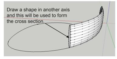
Sophisticated bezier curves can be drawn in Illustrator exported as a DXF and imported into SketchUp Pro. These can be used with the Follow Me tool to produce curved surfaces.
